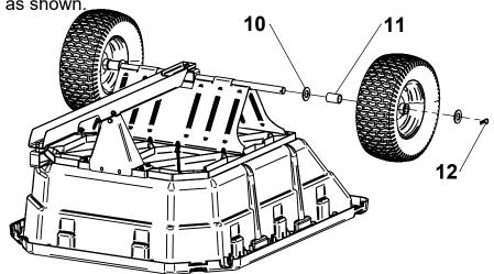
6 Cart assembly is now complete. Check tire pressure regularly and ensure that all hardware is tight prior to use.
