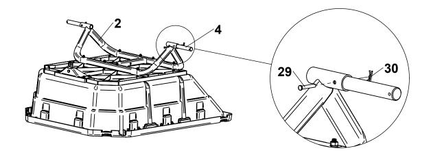
Slide Washers (31), Spacers (35), and Wheels (5) onto Stub Axles (4) and install Cotter Pin (32). Bend legs of Cotter Pin (32) to secure Wheel (5).
