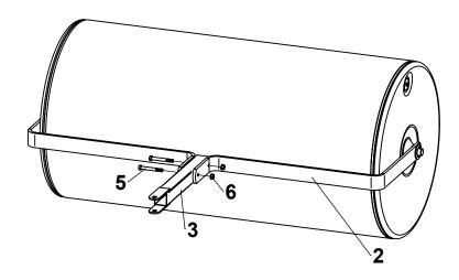
Add Hitch Pin (9) into clevis of Hitch Weldment (3) and secure with Hairpin Cotter (10).
