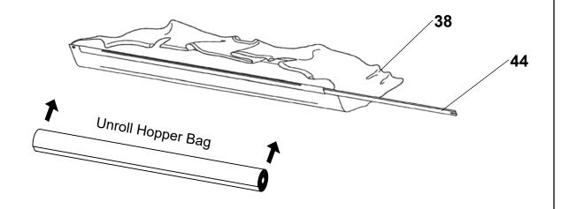
First, place bottom frame assembly into bottom of Hopper Bag (38). Second, Install Clevis Pins (46) through Hopper Bag (38), Hopper Stop Bar (42), and Bottom Frame Tubes (39) then secure with Hairpins(49).
