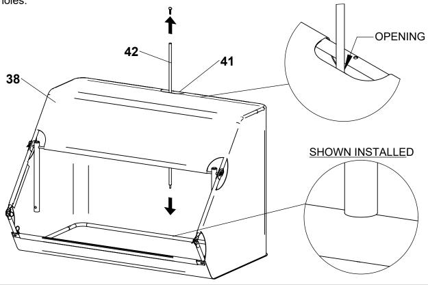
Insert thumb screw that came with Tension Tube Assembly (44) through top Center Frame Tube (41) and screw into top of Tension Tube. Secure Hopper Bag around Top Frame Tubes with Velcro tabs.
